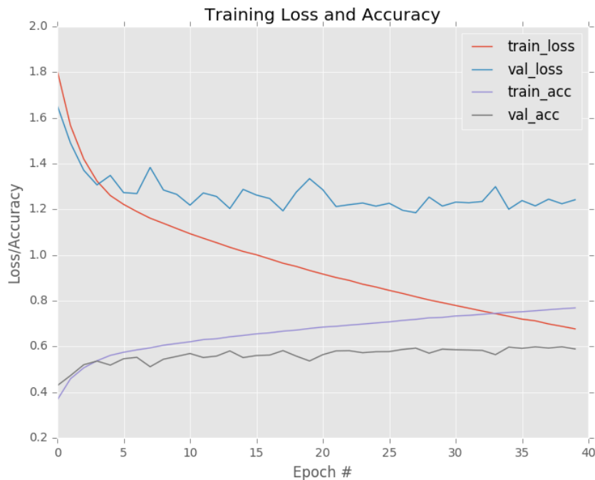
Figure 12.3: Loss and accuracy for ShallowNet trained on CIFAR-10. Our network obtains 60% classification accuracy; however, it is overfitting. Further accuracy can be obtained by applying regularization, which we'll cover later in this book.
