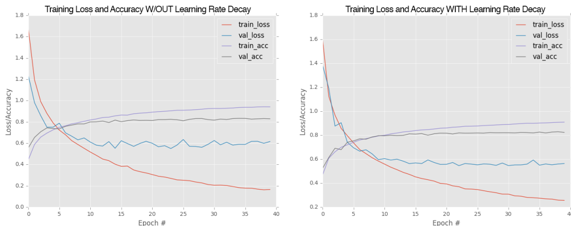
Figure 16.1: Left: Training MiniVGGNet on CIFAR-10 without learning rate decay. Notice how loss starts to increase past epoch 25, indicating that overfitting is happening. Right: Applying a decay factor of 0.01/40 . This reduces the learning rate over time, helping alleviate the affects of overfitting.
