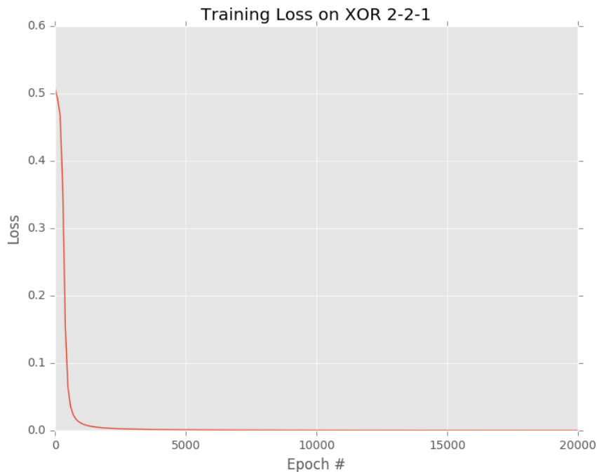
Figure 10.11: Loss over time for our 2 – 2 – 1 neural network.
