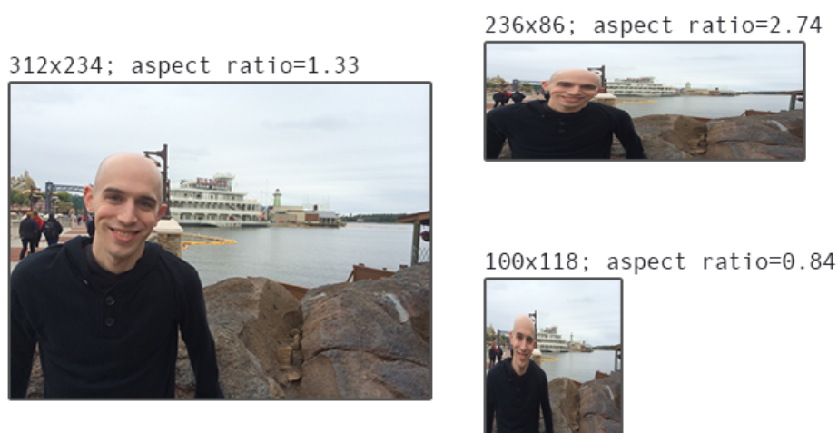
Figure 3.8: Left: Original image. Top and Bottom: Resulting distorted images after resizing without preserving the aspect ratio (i.e., the ratio of the width to the height of the image).
