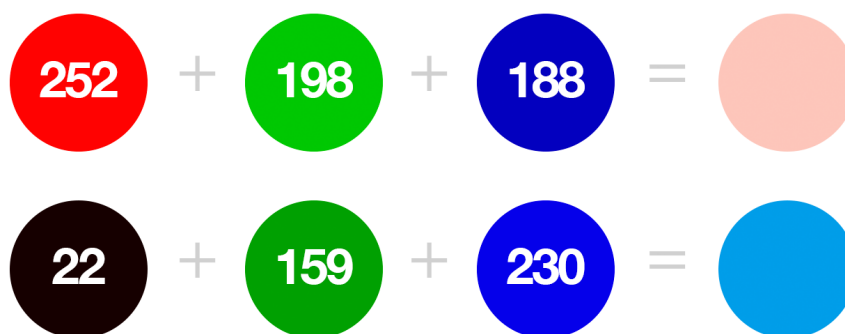
Figure 3.4: Top: An example of adding various Red, Green, and Blue color components together to create a "caucasian flesh tone", perhaps useful in a skin detection program. Bottom: Creating the specific shade of blue in the "PyImageSearch" logo by mixing various amounts of Red, Green, and Blue.
