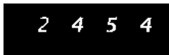
Figure 21.3: Thresholding the image ensures the foreground is white while the background is black . This is a typical assumption/requirement when working with many image processing functions with OpenCV.
