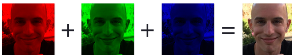
Figure 3.5: Representing an image in the RGB color space where each channel is an independent matrix, that when combined, forms the final image.
