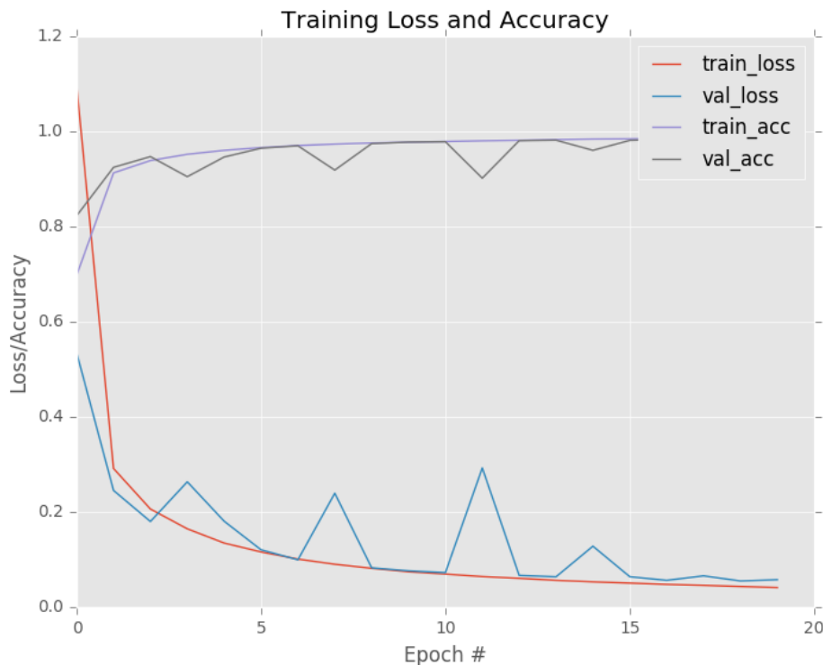
Figure 14.2: Training LeNet on MNIST. After only twenty epochs we are obtaining 98% classification accuracy.
